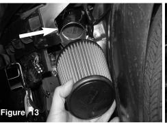
Install the filter to the lower intake tube and then secure the clamp on the filter.
