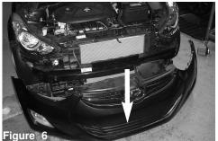
Removal of the front bumper skin will be necessary to install this intake system. There will be a few clips and screws that needs to be remove. If you dont feel comfortable with this procedure, please have your intake installed by a professional
