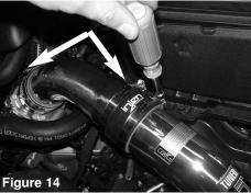
Position for best fit and tighten the remaining clamp using 8mm nut driver.
