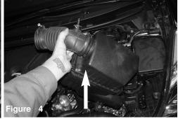
First detach the crank case line. Next loosen the clamp on Now lift up and remove the stock intake assembly from the vehicle.
