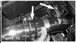
Place the 3.00" straight hose and two clamps onto the end of the upper tube from figure 11 Then position the lower intake tube and align the bracket to the vibra mount and to the straight hose. Place a M6 nut and washer onto the bracket and secure the bracket to the vibra mount. Do not tighten clamps yet.
