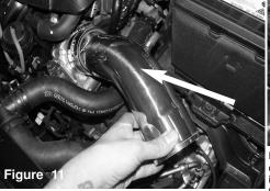
Install the upper intake tube assembly onto the Throttle body. The pipe will require adjustment so do not tighten the clamps yet.
