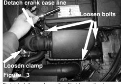
the throttle body and then loosen three bolts attached to
