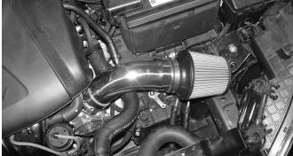
This intake system can be converted short ram for emergency situations.
