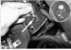
Install the vibra mount to threaded insert on the chassis in the engine bay behind the drivers side headlight. Secure the vibra mount and tighten
