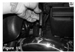
Now secure the crank case line to the fitting on the intake
