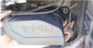
Use the long stud end of the vibra mount to secure the Injen reservoir bottle to the chassise. Continue to secure the other two remaining bolts
