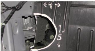
Once the tank has been removed cut a 4" x 5" open on both sides of the splash guard. This will allow access to the bumper area for the filter.
