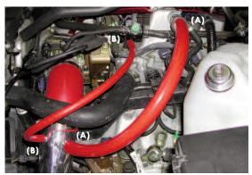
Take the 18" 17mm hose and press one end over the crank case port and the other end over the 3/4" port on the intake(A). The 20" 8mm hose has been connected to both ports (B).
