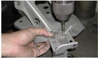
Remove the battery tray from the engine bay. Flip the battery tray upside down and drill out the two spot welds securing the harness bracket to the battery tray.
