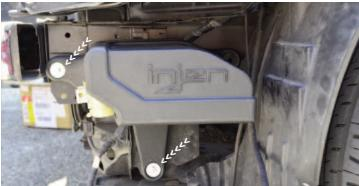
Use 2 MX25 and 2 fender washer to mount the injen reservoir to the chassis. Do not secure the bolts, leave them hand tight for now
